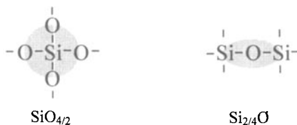
Fig. 1: Two types of structural units describing short- and middle- range order in silicon dioxide matrix.
